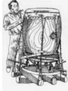
Figure 4: Hydraulic jacks are used to stretch the head of the drum on to its shell.
