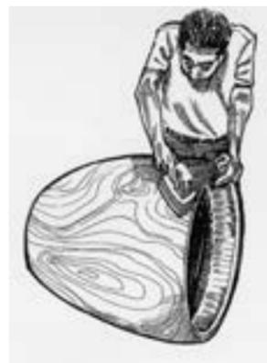
Figure 2: The outside of the drum is sanded for staining.
