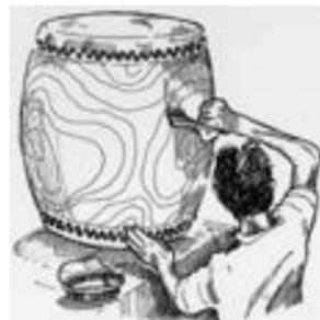
Figure 6: The final step is staining the outside of the drum
