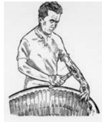
Figure 1: The inside of the bearing edge is chiseled out with a deep-grooved chisel.
